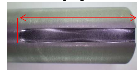
Groove processing by \phi 4 end mill
