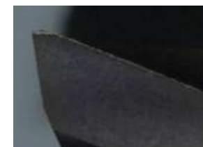
Wear status at the cutting edge
